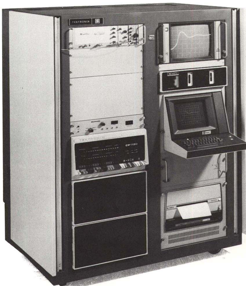
The WP 2000-Series WDI analysis configurations are designed to acquire waveforms of transient phenomena and immediately perform full analyses. Other WDI analysis configurations include from 1 to 32 R7912
