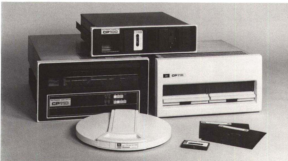
Storage medium options include: 1) dual tape cassette drives, 2) cartridge disk drives and 3) dual floppy disk drives. (Dual floppy disk drives are components
