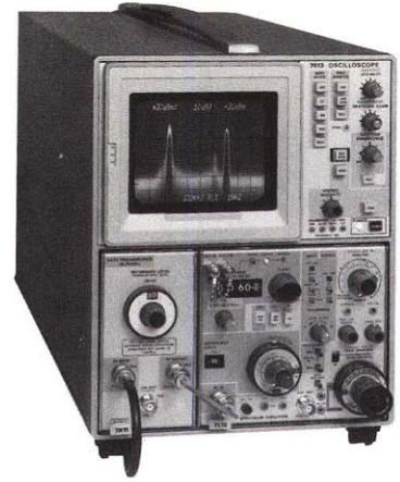
Fig 13. 7K11 Preamplifier Plug-in next to a 7L12 to increase the measurement sensitivity.
