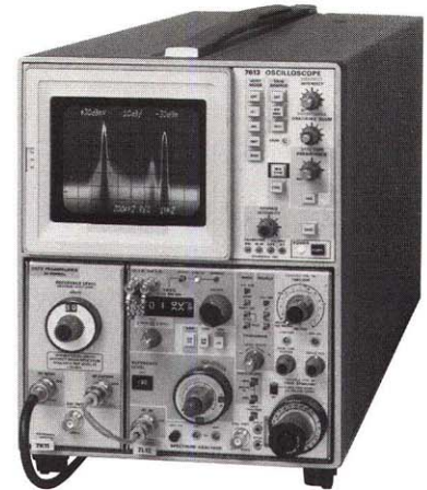
The 7L12 is shown in a 7613 Variable Persistence Mainframe with 7K11 CATV Preamplifier for extra sensitivity.
